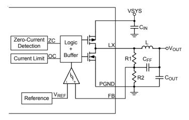
Figure 11. Step-down Converter Block Diagram
