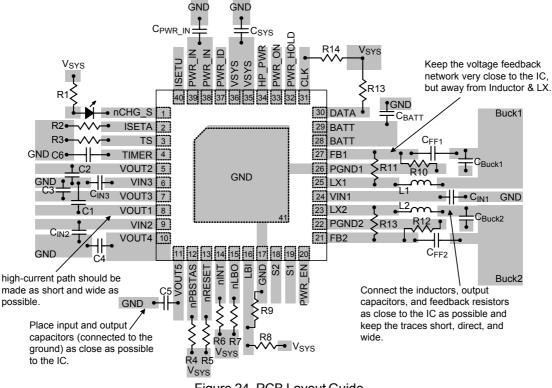
Figure 24. PCB Layout Guide
