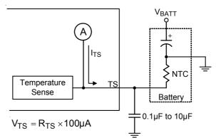
Figure 19. Connection of Battery Temperature Monitor
