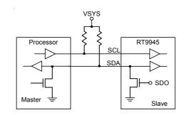
Figure 2. I<sup>2</sup>C Function Block in the RT9945
