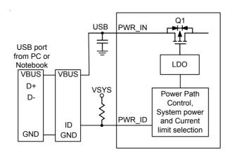
Figure 18. RT9945 Powered by USB port
