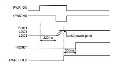
Figure 10. PWR\_ON & HP\_PWR & nPBSTAS Timing Diagram
