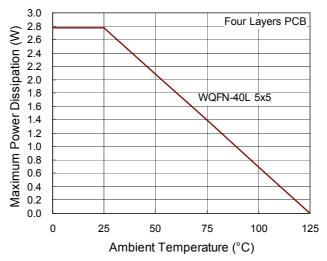
Figure 23. Derating Curves for RT9945 Packages
