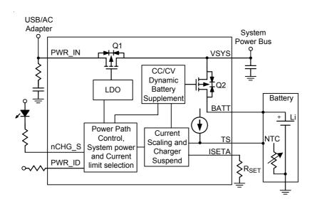
Figure 12. Charger Block Diagram and Required External Components
