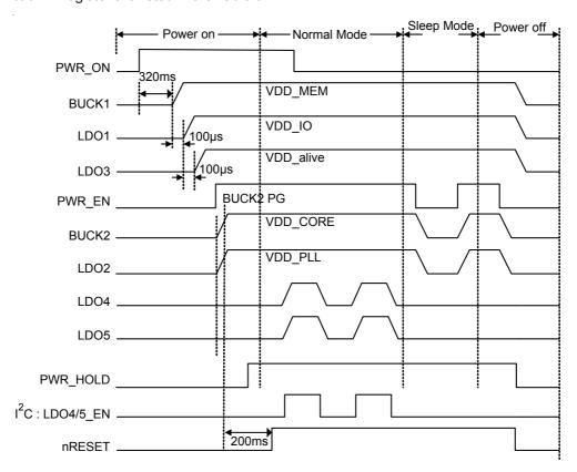
Figure 7. RT9945 POWER ON/OFF Timing Diagram
