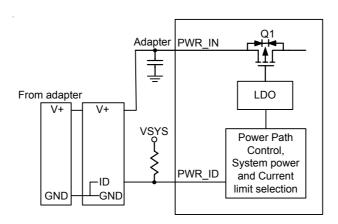
Figure 17. RT9945 Powered by AC Adapter
