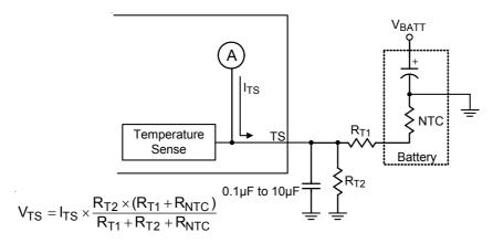
Figure 20. Connection of Battery Temperature Monitor
