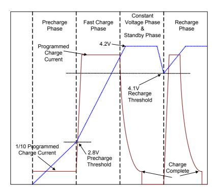
Figure 13. Typical Charge Profile
