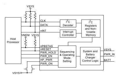
Figure 6. Power and Interface Module
