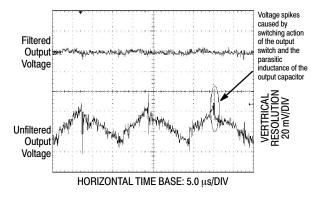
Figure 22. Output Ripple Voltage Waveforms
