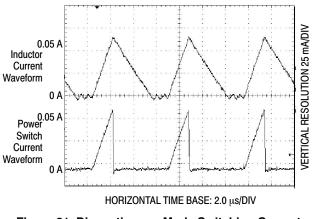
Figure 21. Discontinuous Mode Switching Current Waveforms
