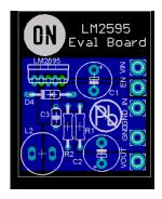
NOTE: Not to scale. Figure 34. Printed Circuit Board Layout Copper Side
