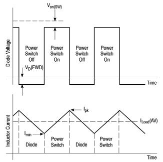
Figure 18. Buck Converter Idealized Waveforms
