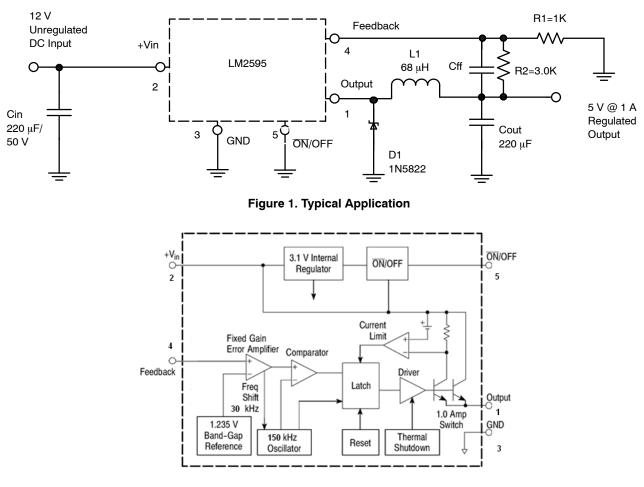
Figure 2. Representative Block Diagram
