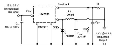
Figure 23. Inverting Buck-Boost Develops -12 V
