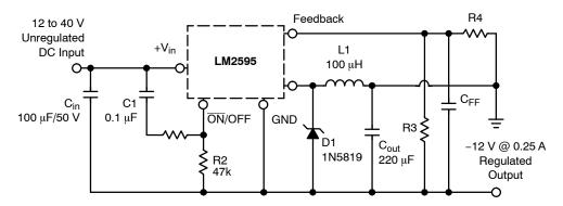
Figure 24. Inverting Buck-Boost Develops with Delayed Startup
