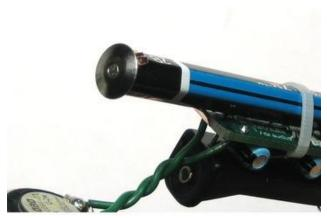
Then take the thumbtack and gently push it into the end of the pencil. You might have to twist it back & forth a little to get it all the way in. The thumbtack will grip the copper tape and also make contact with the graphite in the middle of the pencil to make the first half of the drawing sensor.
