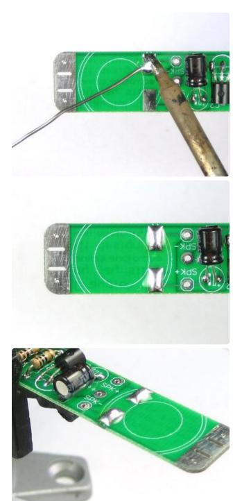
Now melt a lot of solder onto the two pads.
