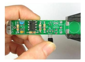
Next is the transistor amplifier Q1 which is PNP type
