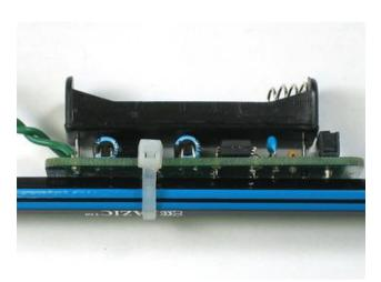
You can mount the drawdio to your pencil. Place the PCB on the flat side of a pencil, and thread the zip tie through as shown and tighten it. You'll want it about an inch or less from the top of the pencil. The higher it is the more pencil you'll have to sharpen but it may be a little more unbalanced.
