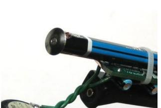
Wrap the tape along the top of the pencil so that the beginning is at the silver metal tab on the PCB, as shown.
