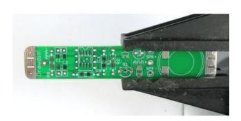
Get ready by placing the PCB in a vise.
