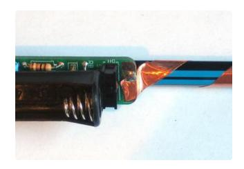
Solder the copper tape to the tab directly as shown.
