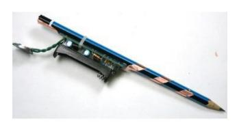
Finally, insert a battery into the kit. Then grip the pencil with one hand and touch the point of the pencil to your other hand. You will be able to hear the drawdio make noise!
