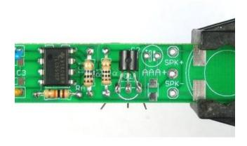
Now bend over the transistor so its 'face flat' against the PCB.
