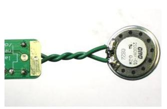
Solder the wires into place.
