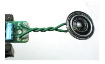
Twist the wires, this will reduce the strain on the solder joints when bending. Put the end of each wire into the two PCB holea marked SPK+ and SPK-. Don't solder into the hole in the middle which is for the battery. The speaker is 'symmetric' so it doesnt matter which wire goes in which hole.
