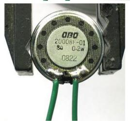
Next, warm up the tabs and slide the tinned ends of wire into the melted solder pool. Then remove the iron and wait a few seconds, the solder pool will cool with the wire in place. Do the same for the other pad.
