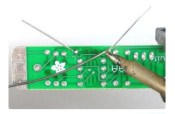
Turn the PCB over. Using your soldering iron tip, press and heat both the pad (the silver ring around the hole) and lead (wire) at the same time for 2 or 3 seconds. Then poke the end of the solder in to create a nice solder joint. Do this for both leads.
