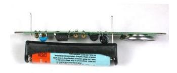
Slide the battery holder into the PCB (but do not solder it in). Make sure that the battery is aligned correctly. Putting in the battery backwards shouldn't damage the circuit but it's still not a good idea so try to get it right the first time. The back of the PCB has a silkscreen to help determine which way the battery goes in.
