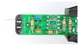
Next are the two ceramic capacitors C1 andC3. Ceramic capacitors also have a nice property that they are symmetric/non-polarized. That means they can go in 'either way'. The capacitors are different values so make sure to not mix them up.
