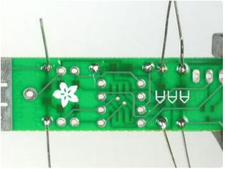
Once you are positive about R1 and R2, solder in these resistors using the same technique you used for the first resistor.
