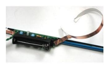
Next take 3 or 4" of copper tape and start wrapping around the bottom of the pencil, starting with the silver tab on the PCB and ending an inch before the end of the pencil. This will make contact with your hand and provide the second half of the sensor.
