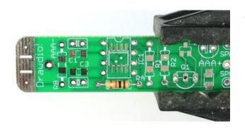
Bend the resistor into a staple as shown, and slip it in.
