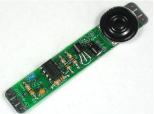
Now use the tip of your iron to quickly remelt the blobs so that they flow onto the speaker tabs.
