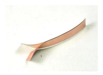
Next cut a 1.5" piece of copper tape using the diagonal cutters. Don't use scissors as the metal tape can damage them. Peel off the paper backing. The copper tape is conductive, sticky and flexible which makes it perfect for wrapping the pencil.
