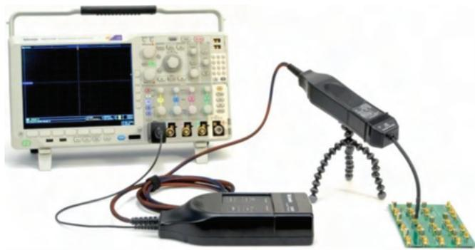
Figure 4: Tektronix IsoVu measurement setup.
