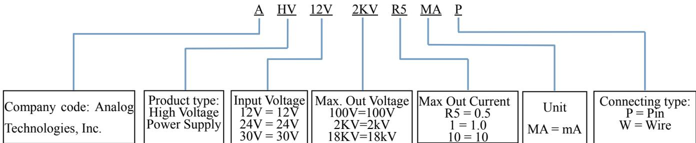
Figure 10. Naming Principle of AHV12V2KVR5MAP
